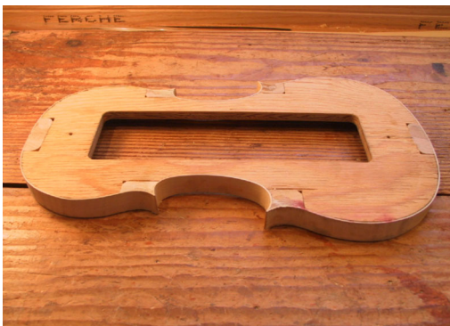
On this soprano violin, the spacing aligns the mold with the surface of the blocks.
