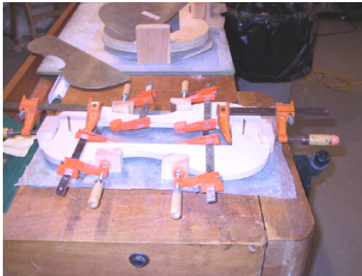
On this alto violin, the spacing of the mold to align with the center of the blocks can be seen. The same for the cello in the rear.
