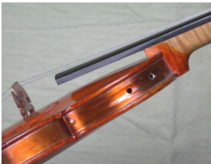
Prototype treble violin showing varnished aluminum ribs with hand-filed groove and riveted corner.
